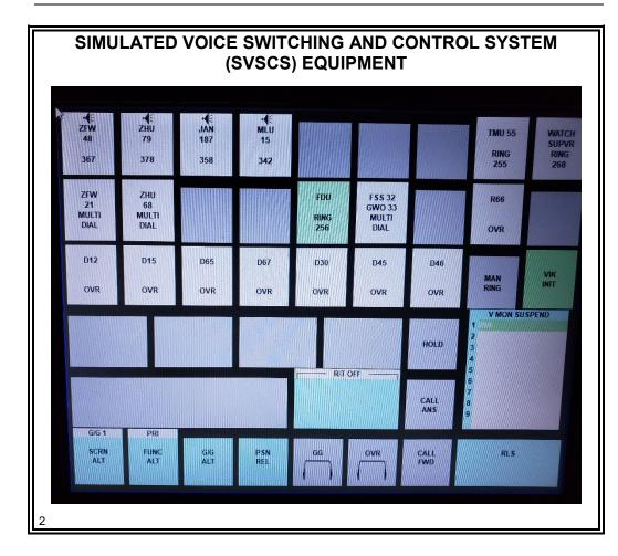
In en route facilities, the Voice Switching and Control System (VSCS) provides air traffic controllers with Air-to-Ground (A/G) and Ground-to-Ground (G/G) voice communication capability. VSCS interfaces with remote radio equipment and facilitates voice connectivity between controllers within the same facility as well as separate facilities. Knowledge of the VSCS is vital for your progression to Certified Professional Controller (CPC).
